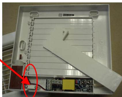
2. Connect the fan with power supply using the terminal strip on electronics. Usually goes from wall electric cable with 3 wires, so the blue is directly earthed conductor (N), brown / black is the phase conductor (L – under constant voltage) and third yellow-green is the circuit protective conductor (no need to connect when mounting plastic fan, can be blinded). Install the fan so the service cables will be in lower part of the fan.
