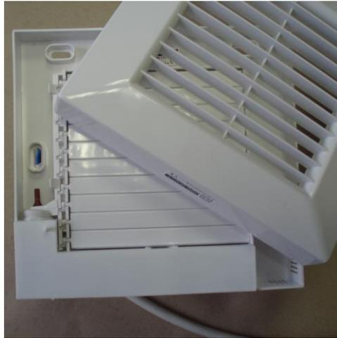
4. Turn on on-off switch to bring power supply 230V/50Hz into device – fan starts to work. At the same time thermoactuator gets warmer and during cca 50 seconds is the shutter open. After switch off device stops. Thermoactuator get colder and closes the shutter (watt cca 2,5 minutes until complete closure).
