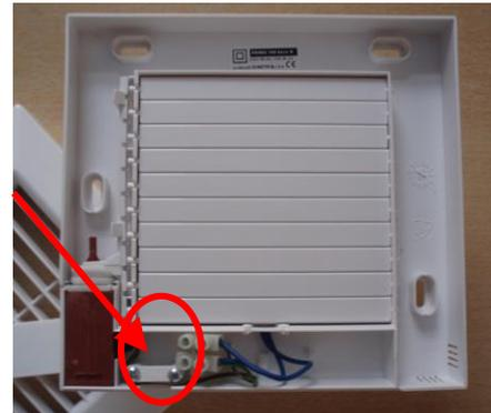
2. Connect the fan with power supply using the terminal strip. Usually goes from wall electric cable with 3 wires, so the blue is directly earthed conductor (N), brown / black is the phase conductor (L – under constant voltage) and third yellow-green is the circuit protective conductor (no need to connect when mounting plastic fan, can be blinded).
